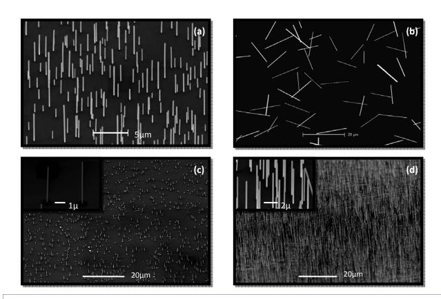
**Figure 2:** SEM images of as-grown Ni NW arrays with (a) vertical orientation grown at 650°C, (b) horizontal orientation grown at 700°C and vertically oriented NWs with (c) low density and diameter near 100nm grown at 630°C and (d) high density and diameter near 250nm grown at 675°C.
