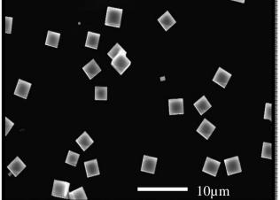
**Figure 1**: Single-crystal Ni cubes formed on SiOx coated Si substrates.
