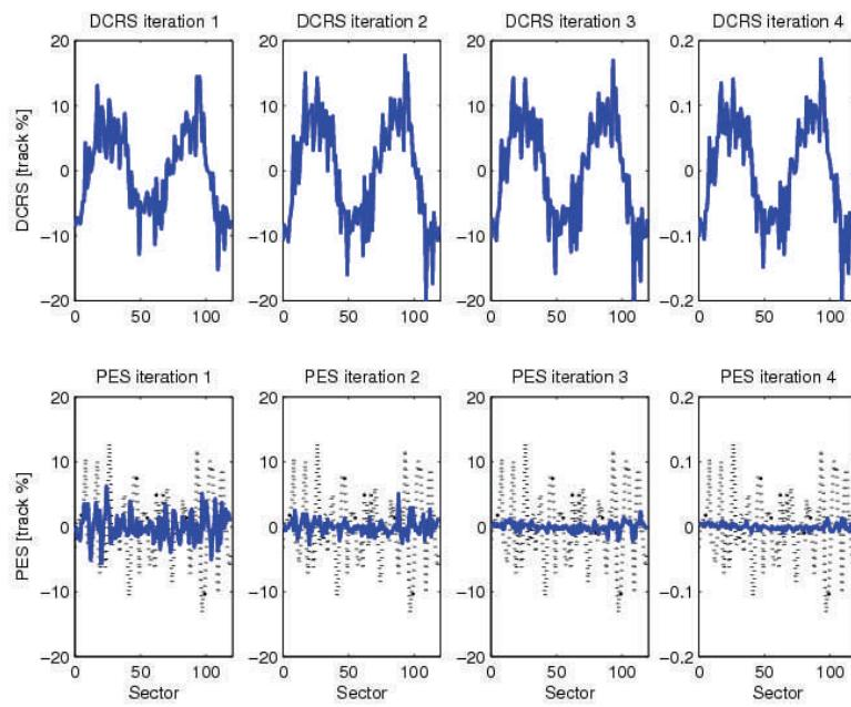
Independently, work funded by several gifts from Headway to the AMSL has unleashed the ability to target specific periodic disturbance (repeatable runout errors) typically seen in the rotating storage media of a HDD. By the development of an Iterative Learning Control algorithm, that only requires limited knowledge of the closed-loop response of a servo actuator, Prof. de Callafon and his student Matthew Graham were able to show in
