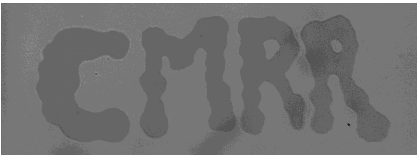
Figure 1 Magnetic image of a saturated [Co(5\text{\AA})/Tb(4\text{\AA})]_{x28} multilayer film, where pulses of circularly polarized light were used to reverse the magnetization of certain areas. The full size of this image is about 100 \mu\text{m} long.
