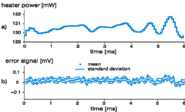
Fig. 14. a) Heater power versus time, and b) error signal versus time while applying the optimal feedforward profile to the heater (average of 20 consecutive disk revolutions).
