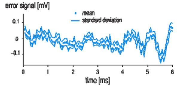
Fig. 10. Error signal versus time for one disk revolution (average of 20 consecutive disk revolutions).
