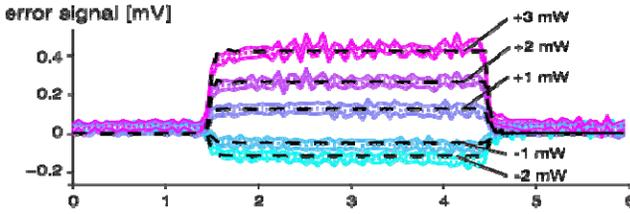
Fig. 11. Comparison between measured and dynamic simulated error signal resulting from rectangular pulses in heater power (average of 20 consecutive disk revolutions).
