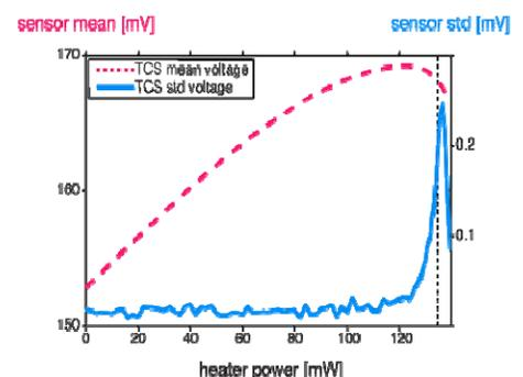
Fig. 4. TCS voltage output versus heater input power. Head-disk contact is detected at 134.5 mW according to the sensor standard deviation (std) as indicated by the vertical dashed line.
