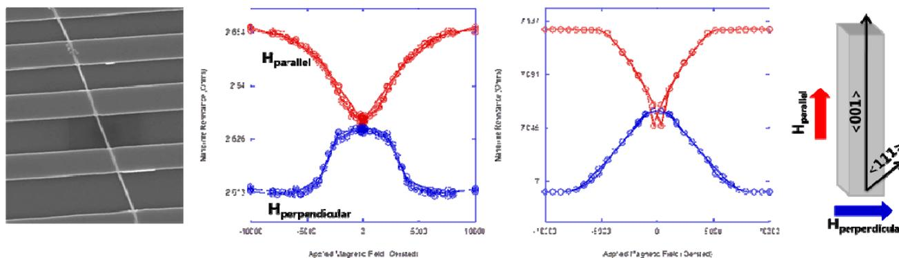
**Figure 3:** We use magneto-transport measurements of individual Ni NWs to probe their magnetic response to field. The left image is an individual wire with leads where we measure the resistance as a function of applied field parallel and perpendicular to the wire axis. The left graph is the measured data and the right graph is the results of micromagnetic simulations.
