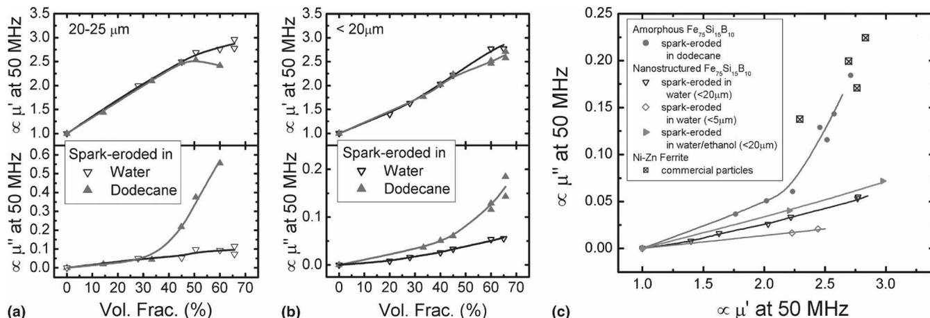
FIG. 9. Permeabilities measured at 50 MHz for composites of particles: (a) 20–25  $\mu\text{m}$  and (b)  $< 20 \mu\text{m}$ , as prepared in dodecane and in water, as functions of particle concentrations; and (c)  $\mu''$  versus  $\mu'$  for composites made from various particles. Composites made with NiZn ferrite particles are included for comparison.
