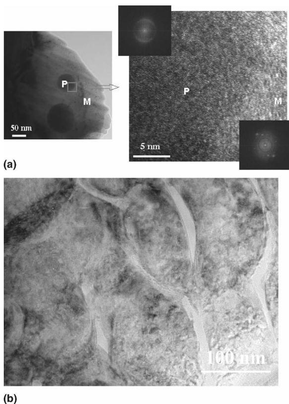
FIG. 4. TEM micrographs of Fe–Si–B particles: (a) spark-eroded in water (insets are selected-area electron-diffraction patterns of an amorphous nanoparticle and the crystalline matrix); and (b) spark-eroded in ethanol. Note the amorphous channels (lighter contrast) separating the crystalline regions.
