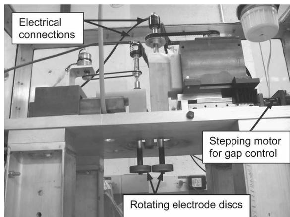
FIG. 1. Photograph of the rotating electrode spark-erosion system with Fe–Si–B disks mounted.
