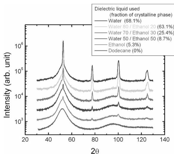
FIG. 3. XRD spectra of Fe–Si–B particles spark-eroded in different water/ethanol mixtures, indicating different proportions of crystalline and amorphous phases. The spectra are ordered as indicated in the inset.
