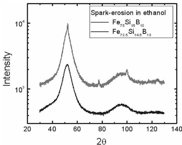
FIG. 6. XRD spectra for Fe–Si–B particles spark-eroded in ethanol using starting alloys with different concentrations, as indicated. The Fe/Si ratio was kept constant for both alloys, while the B concentration was increased by 3%.
