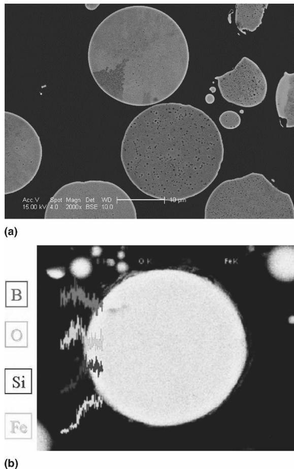
FIG. 5. SEM micrographs of cross sections of particles spark-eroded in water after mechanical polishing. White rings corresponding to oxide surface layers are visible in (a), and variations in local chemical composition indicated by small-probe x-ray microanalysis profiles are shown in (b).
