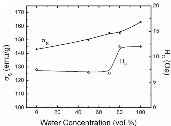
FIG. 8.  $\sigma_s$  and  $H_C$  as functions of water concentration in the water/ethanol dielectric liquid.
