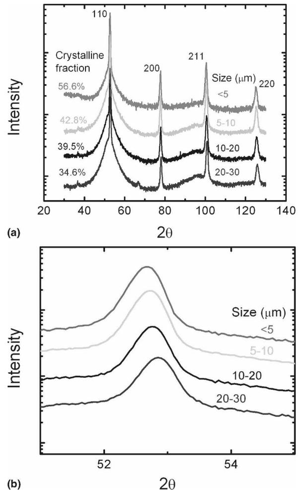
FIG. 7. XRD spectra of Fe–Si–B particles spark-eroded with high power and a large gap to produce particles of various sizes ranging up to ~30 μm. (a) Particles classified by sieving; and (b) magnified view of the 110 peaks shows that the peak position shifts slightly depending on the average particle size.
