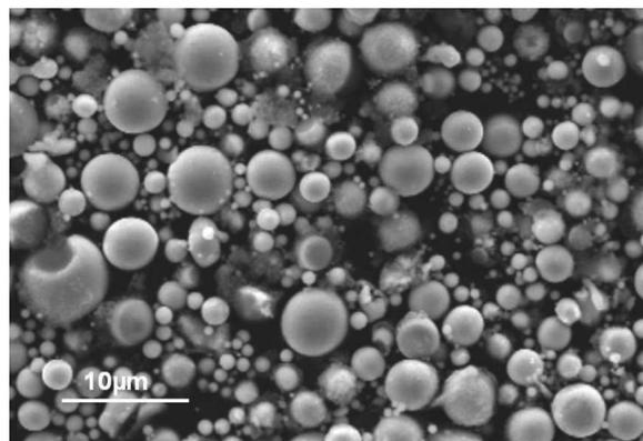
FIG. 2. SEM micrograph showing spherical particles spark-eroded in a water/ethanol (50:50) mixture.
