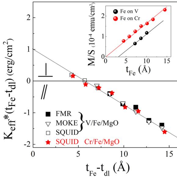
FIG. 3. Effective anisotropy constant  $K_{eff}$  times  $t_{Fe}-t_{dl}$  as a function of  $t_{Fe}-t_{dl}$  deduced from SQUID-VSM, FMR, and MOKE measurements at RT for both V/Fe/MgO and Cr/Fe/MgO systems. The line is a fit using Eq. (2). In inset are plotted the areal magnetization versus Fe thickness, showing that  $t_{dl} = 0$  for Fe on Cr and  $t_{dl} = 3 \text{ \AA}$  for Fe on V.
