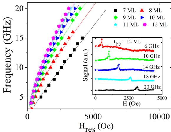
FIG. 4. FMR resonance field plotted versus DC magnetic field frequency (points) and simulations (lines) performed on V/Fe/MgO wedge with  $t_{Fe} = 7, 8, 9, 10, 11,$  and  $12$  MLs. In inset, typical FMR responses versus field for  $t_{Fe} = 12$  MLs for several excitation frequencies of the in-plane applied DC field.
