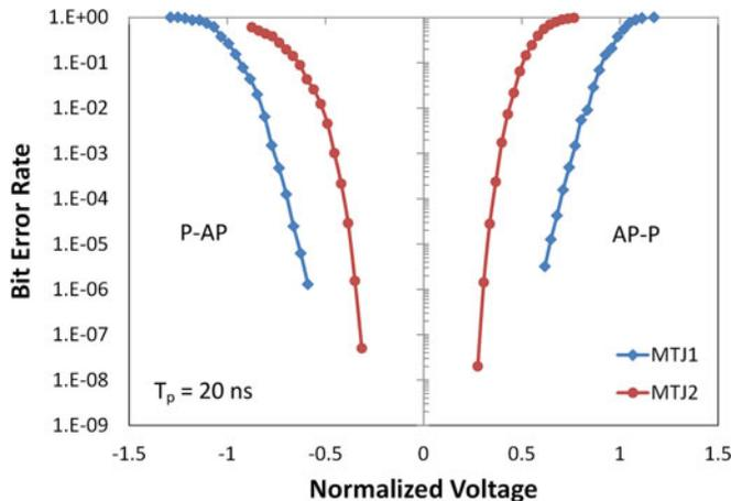
Fig. 1. RDRs of two representative MTJ devices with different free/capping layers. The pulse width is 20 ns.
