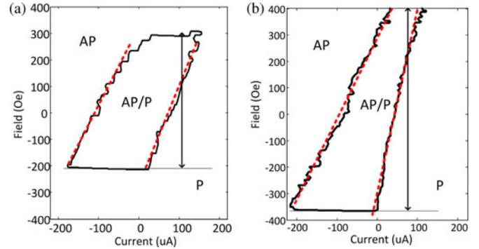
Fig. 7. SSDs of (a) MTJ1 and (b) MTJ2. MTJ2 shows substantially different slopes between AP-P and P-AP switching boundaries, as indicated by dotted lines.
