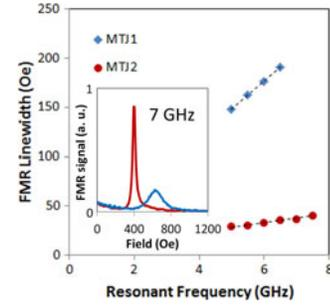
Fig. 6. FMR linewidth versus resonant frequency. The damping constant values of MTJ1 and MTJ2 were 0.007 and 0.037, respectively. The inset shows the FMR peaks measured at 7 GHz.
