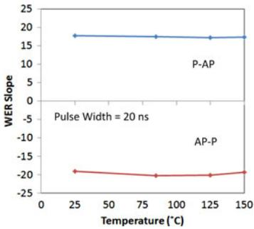
Fig. 5. WER slopes as a function of temperature.
