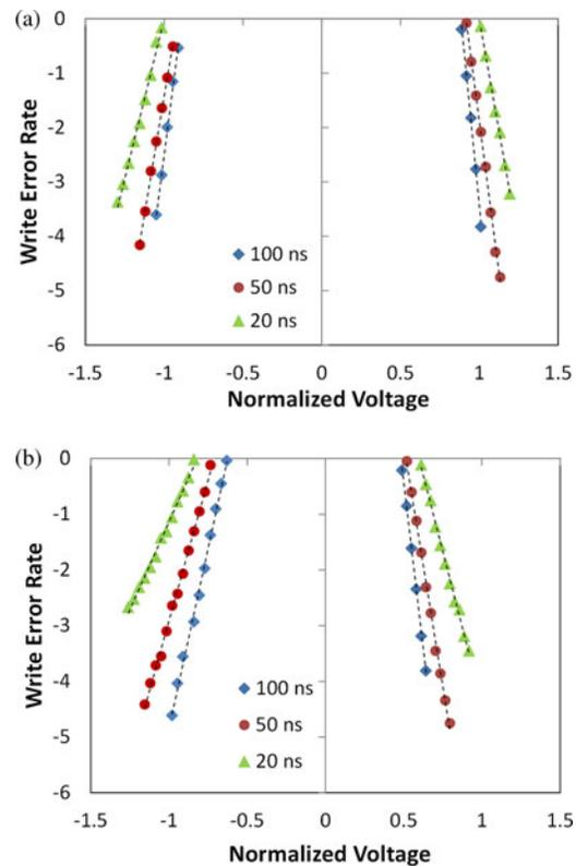
Fig. 2. Normal quantile plots of WERs measured from two representative MTJ devices. (a) MTJ1. (b) MTJ2. Only MTJ2 shows asymmetric WER slopes. Dotted lines are fits to the Gaussian CDF.
