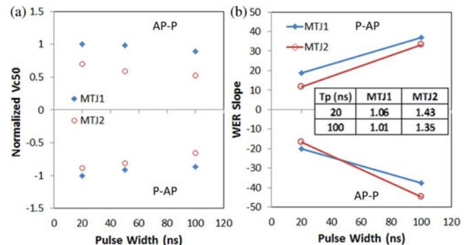
Fig. 3. (a) Normalized  $V_{c50}$  versus pulse width. (b) WER slopes versus pulse width. The data points averaged from >30 MTJs per split. The inset shows WER asymmetry of each split.
