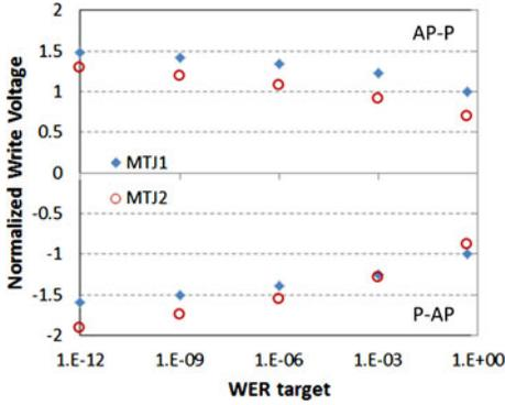
Fig. 4. Write voltage requirement versus WER targets. The write voltage requirement was estimated from the Gaussian CDF fits. This is the average behavior of all the measured MTJs.
