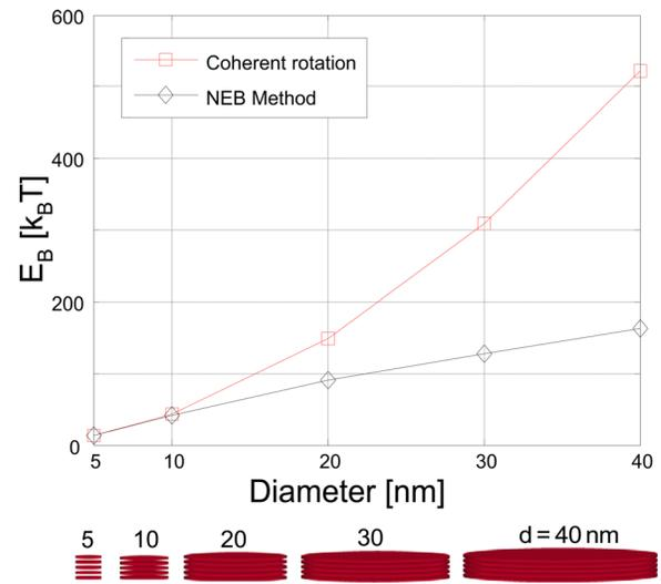
FIG. 3. (Color online) Micromagnetic results for the minimum energy reversal pathway (NEB results) for [Co(0.3 nm)/Pd(0.7 nm)]<sub>5</sub> multilayer islands ranging from 5 nm to 40 nm in diameter compared to the macrospin approximation.
