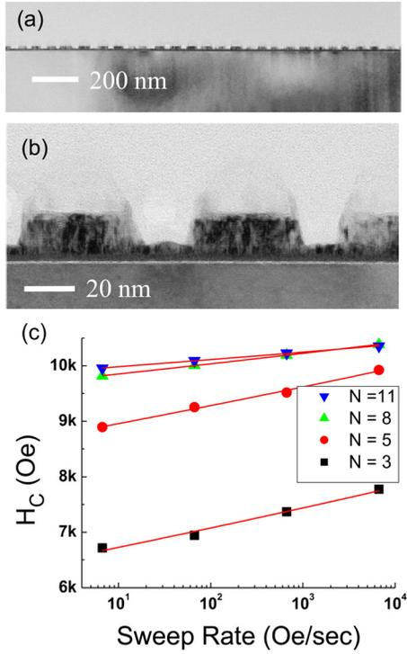
FIG. 1. (Color online) Lower (a) and higher (b) resolution images of patterned  $[\text{Co}(0.3 \text{ nm})/\text{Pd}(0.7 \text{ nm})]_{11}$  multilayers. (c) Time-dependent coercive fields for  $N = 3, 5, 8,$  and  $11$ . The solid lines are fits to Eq. (1) with the fit parameters given in Table I.
