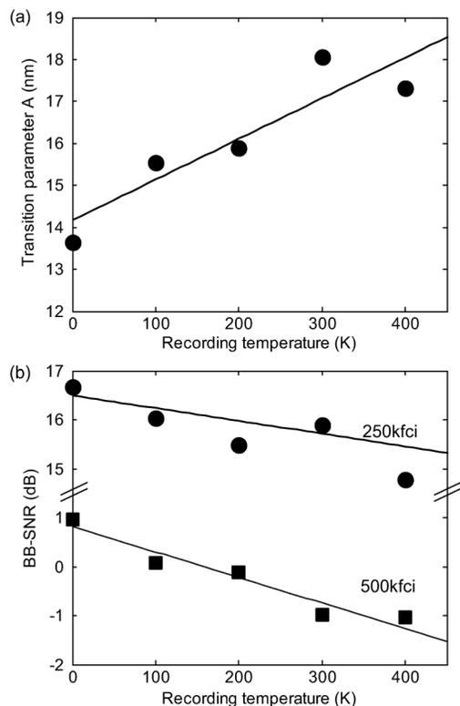
Fig. 4. (a) Variation of the recorded transition parameter versus the recording temperature  $T$ . Dots are simulation results and the line is a linear regression. (b) Variation of BB-SNR values versus  $T$ . Symbols are simulation results and the lines are predictions of the BB-SNR using, for the transition parameter, the linear approximation of Fig. 4(a).
