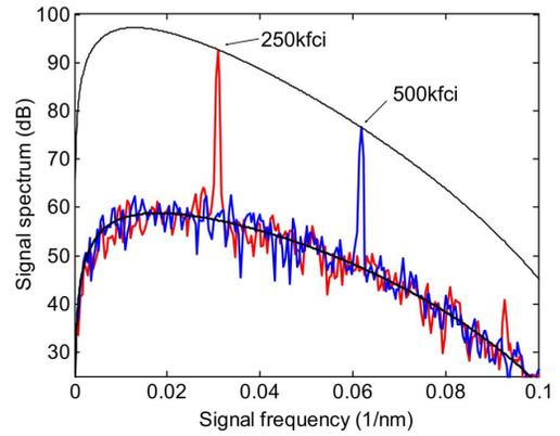
Fig. 3. 250 and 500 kfci signal spectra obtained from simulations performed for a recording temperature  $T = 300$  K. Lines are signal roll-off fit ( $d + a = 43$  nm) and noise spectrum fit ( $d = 24$  nm).
