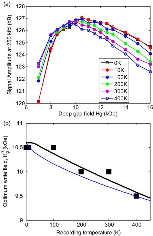
Fig. 2. (a) Signal amplitude at 250 kfci versus writer deep-gap field for different recording temperature. (b) Optimum writer field  $H_g^0$  as a function of the recording temperature. Black line is  $H_g^0(T)$  calculated from Eq. (3) with  $R = 2e11$  Oe/s. Fine blue line is  $H_g^0(T)$  calculated from Eq. (2) with  $t_{eff} = 3$  ns.
