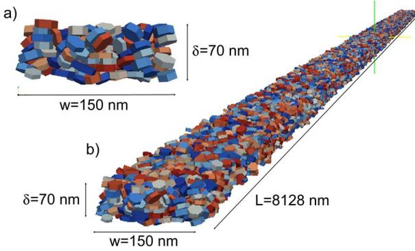
Fig. 1. Illustration of a, 8- $\mu\text{m}$ -long, 150-nm-wide, 70-nm-thick BaFe particulate media slab used in the write simulations. (a) Side view, (b) perspective view.
