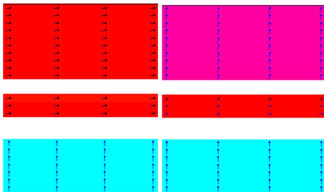
FIG. 5. Switching diagram for the IEC parameters  $0.5 \text{ erg/cm}^2$  (left) and  $0.05 \text{ erg/cm}^2$  (right) at the current density  $7 \times 10^6$  A/cm<sup>2</sup>. Bottom layer is the polarizer layer, middle layer is the CoFeB layer with interfacial anisotropy and top layer is the Co/Pt-ML with bulk anisotropy.
