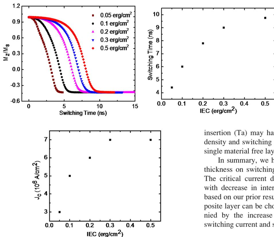
FIG. 3. (a) Magnetization switching for different exchange parameters at the constant current density  $7 \times 10^6$  A/cm<sup>2</sup>. (b) Switching time as a function of exchange parameter.
