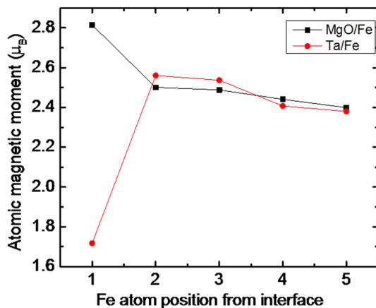
FIG. 1. Atomic magnetic moment behavior for the Fe atoms near the interfaces with MgO and Ta.
