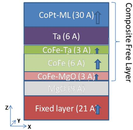
FIG. 2. The cartoon of the modeled stack.
