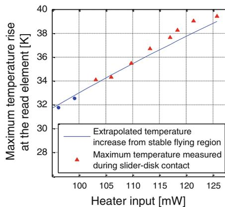
**Fig. 10** Maximum temperatures measured during slider-disk contact and extrapolated temperature increase from the stable flying region below 103 mW to the unstable flying region above 99 mW for a constant heater input profile
