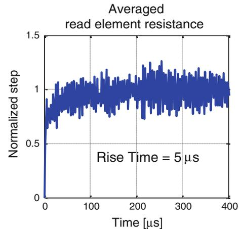
**Fig. 12** Averaged normalized response time of the read element for a square wave heater input with a step size of 1 V
