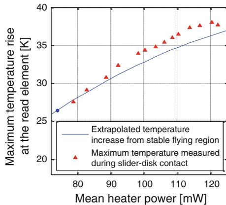
**Fig. 11** Maximum temperatures measured during slider-disk contact and extrapolated temperature increase from the stable flying region below 74 mW to the unstable flying region above 74 mW for a square heater input profile
