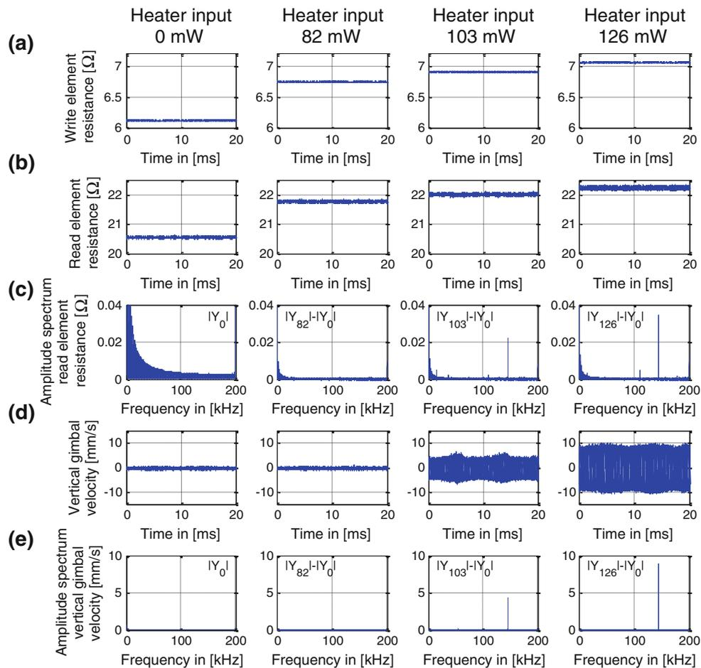
**Fig. 2** **a** Write element resistance, **b** read element resistance, **c** change in frequency spectrum of the read element resistance after subtracting the resistance spectrum  $|Y_0|$  at 0 mW, **d** vertical gimbals velocity and **e** change in frequency spectrum of the vertical gimbals
