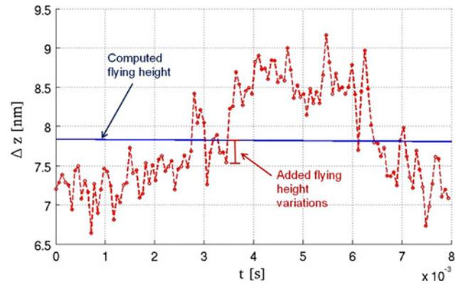
Fig. 5 Flying height variations (dotted points) were added to the computed steady state flying height (solid line) to simulate a flying height profile (dash line)
