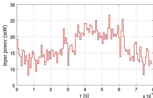
Fig. 7 Heater element power input time dependent history
