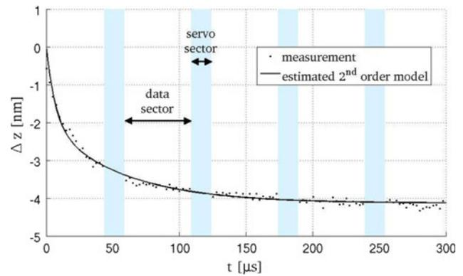
**Fig. 2** Flying height change  $\Delta z$  due to a step power input to the heater element. Source: Boettcher et al. (2011)
