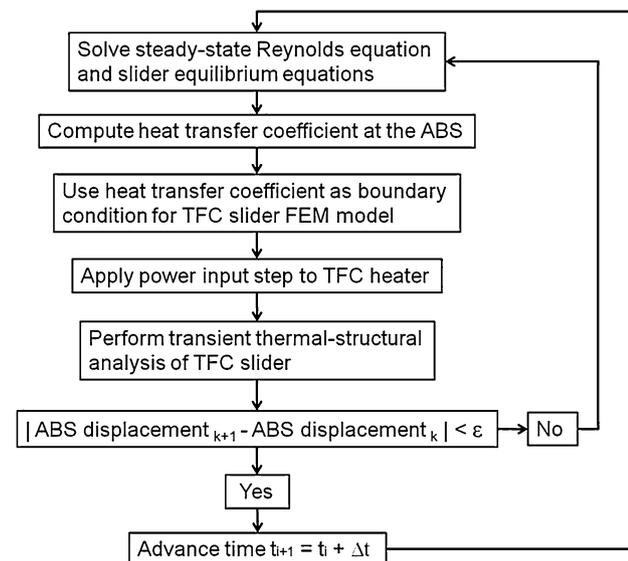
Fig. 4 Schematic representation of time dependent simulation of TFC slider response
