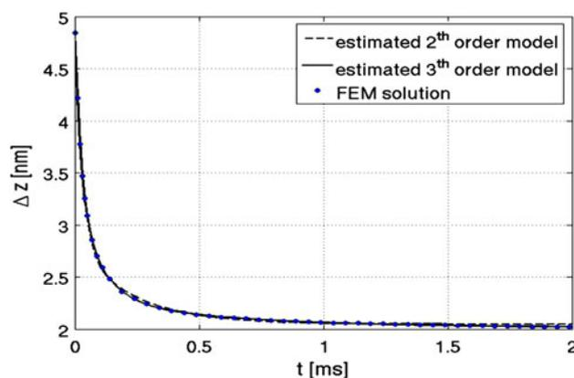
Fig. 6 Computed and estimated time dependent flying height history for a power input step
