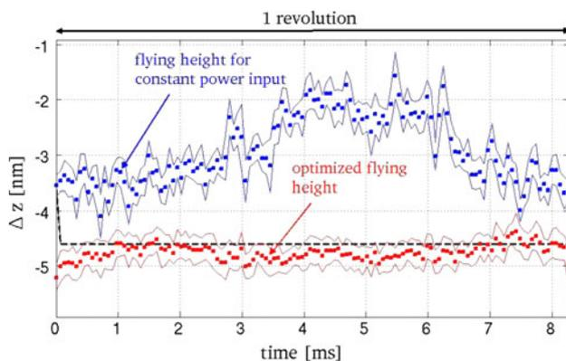
**Fig. 1** Experimentally measured flying height profiles due to constant and optimized power input to the heater element. The square symbols represent the mean of 20 measurements. The solid lines represent one standard deviation confidence intervals for each set of measurements. Source: Boettcher et al. (2011)
