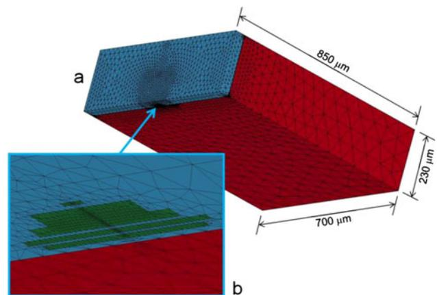
**Fig. 3** Finite element model of (a) TFC slider and (b) read-write element
