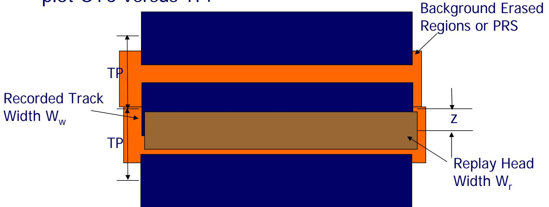
$z$  is off track displacement, TP is cross track center to center distance between adjacent tracks.
