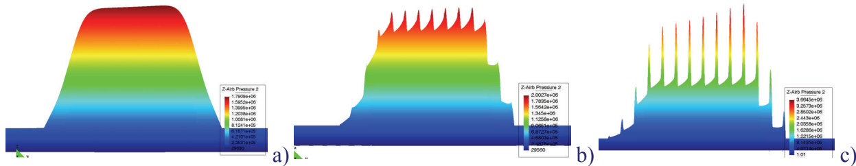
Fig. 2 Trailing edge center pressure distribution for a) smooth disk, b) 15nm groove depth, c) 75nm groove depth.
