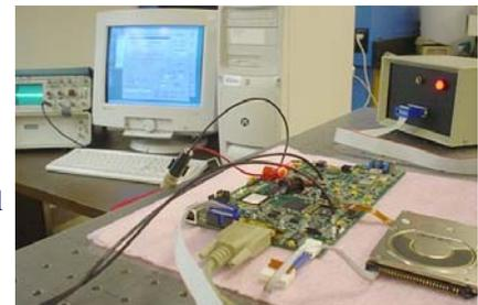
procedure that allows estimation of models for actuator and disturbance dynamics, whereas collaborative work with Prof. Oboe [2] has shown the successful implementation of this procedure on actual data obtained from a HDD system.
