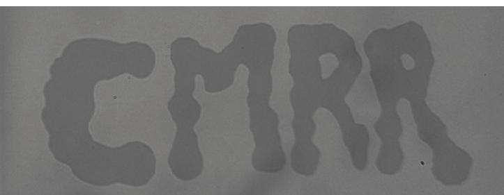
Figure 1: Magnetic image of a saturated  $[Co(5\text{\AA})/Tb(4\text{\AA})]_{x28}$  multi-layer film, where pulses of circularly polarized light were used to reverse the magnetization of certain areas. The full size of this image is about 100 mm long.
