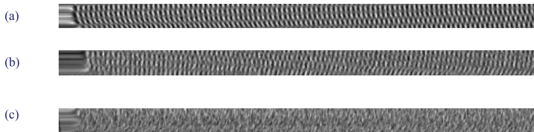
Fig.1. SMRM images of 4200 Oe hard disk media. (a) original 72.5 MHz pattern; (b) after partial erasure; (c) after complete erasure.
