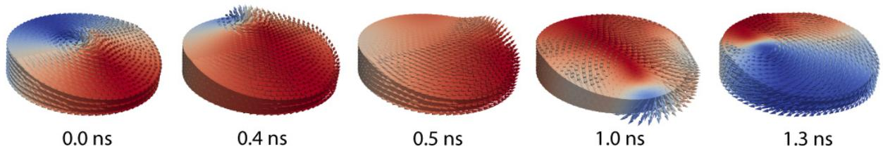
*Fig. 1 Temporal evolution of the magnetization circulation switching in a 100-nm-wide nanodisk by a 0.5-ns-long magnetic field pulse applied in the disk plane (micromagnetic simulation in the finite-element FastMag code [11]). Snapshots show the instantaneous magnetization configuration at indicated time delays.*
