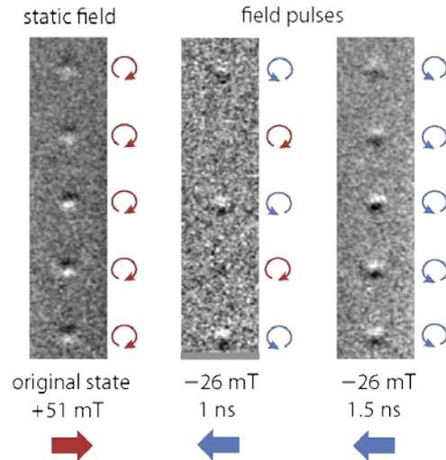
Fig. 3 The MTXM images of vortices in 250-nm-wide and 20-nm-thick disks were taken after application of in-plane magnetic fields. The arrows on the right of each image indicate spin circulation. Arrows and labels below the images show the polarity and magnitude of the applied field, as well as pulse duration where applicable.
