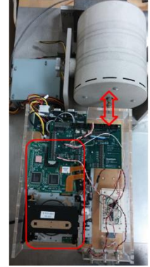
Fig.1: Vibration setup with LTO drive on shaker table.
